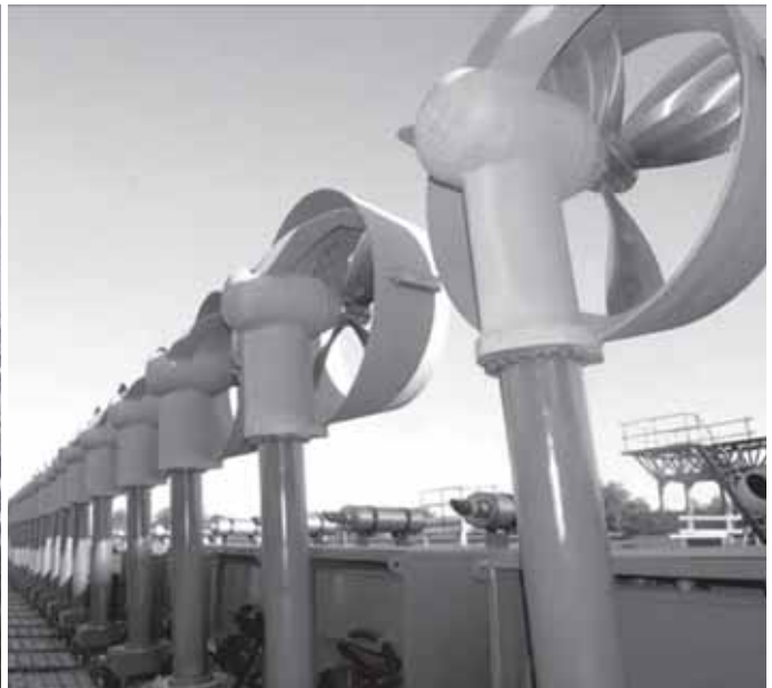
Self-contained thruster packages for main propulsion and positioning of barges, platforms and river craft.
